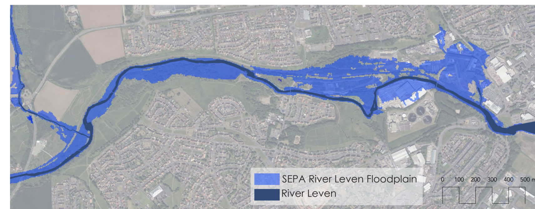
The floodplain SEPA mapping shows the natural extent of flooding for an extreme event (200 year return period plus climate change). We must not do anything within the floodplain that reduces flood storage.
